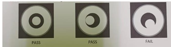
Figure 7. Standard limit for light beam deviation
